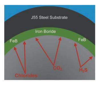
The EndurAlloy surface is comprised of one atom of boron and one atom of iron, which combine to create a molecule of iron boride. EndurAlloy provides excellent corrosion resistance because it is inert\ and non-reactive to most of the corrosive elements found in oil and gas production.
